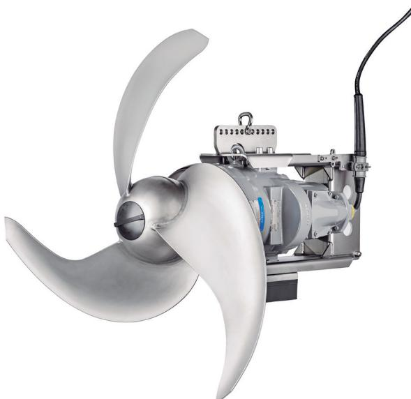
Xylem presented the Flygt 4530 model, featuring a highly efficient 1.2 metre diameter stainless steel propeller and a propeller speed of just 108 revolutions per minute. This gives it high thrust in relation to power consumption. High thrust is essential to keep sludge and everything else in suspension, thus preventing deposits that slowly decrease the efficiency of the process, whilst also reducing the frequency with which the tank needs to be cleaned.
